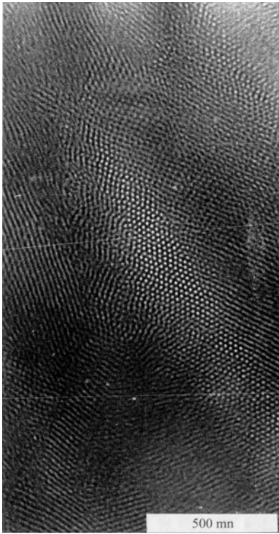
Fig. 3 TEM micrograph of I_{37}B_{37}S_{20}^{70} stained with OsO_4 (polystyrene domains appear bright)
