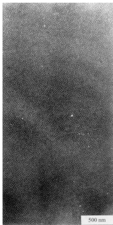
Fig. 2 TEM micrograph of I_{46}B_{38}S_{16}^{74} stained with OsO_4 (polystyrene domains appear bright)
